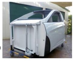
Paul sources the vehicles from local motor wreckers and then constructs them in his garage at home. He has designed and drawn the plans and then undertakes the task of building them. The car is able to be set at different heights so that the user will be able to enter and exit all types of modern vehicles.
